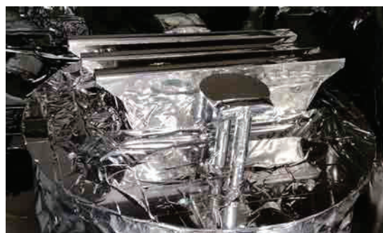
Fig.1 Photograph of three parts of ellipsoidal neutron supermirrors coated by the ion beam sputtering instrument (KUR-IBS) at KURNS.
