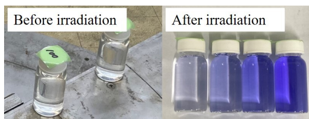
Fig. 1. An example of color change before and after the irradiation using the LCV micelle gel dosimeters.
