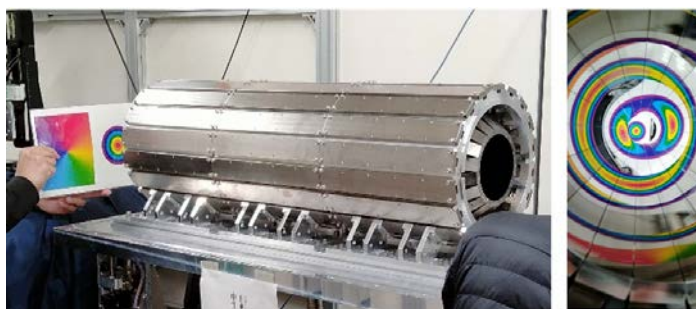
Fig.1 Photograph of a full circumference, ellipsoidal neutron supermirror made of 54 mirror pieces.
